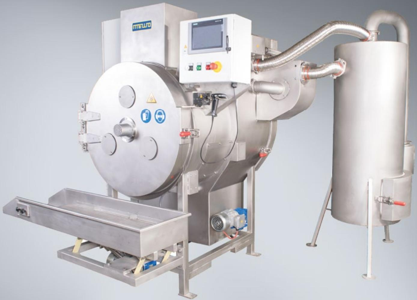
The JET ROTOR-Series is a very powerful basic drum-type media-blasting deburring system. It is an ideal introduction for the cryogenic finishing of rubber, plastics and non-ferrous metals from small to medium sized batches. It has a batch volume of up to 50 litres.
