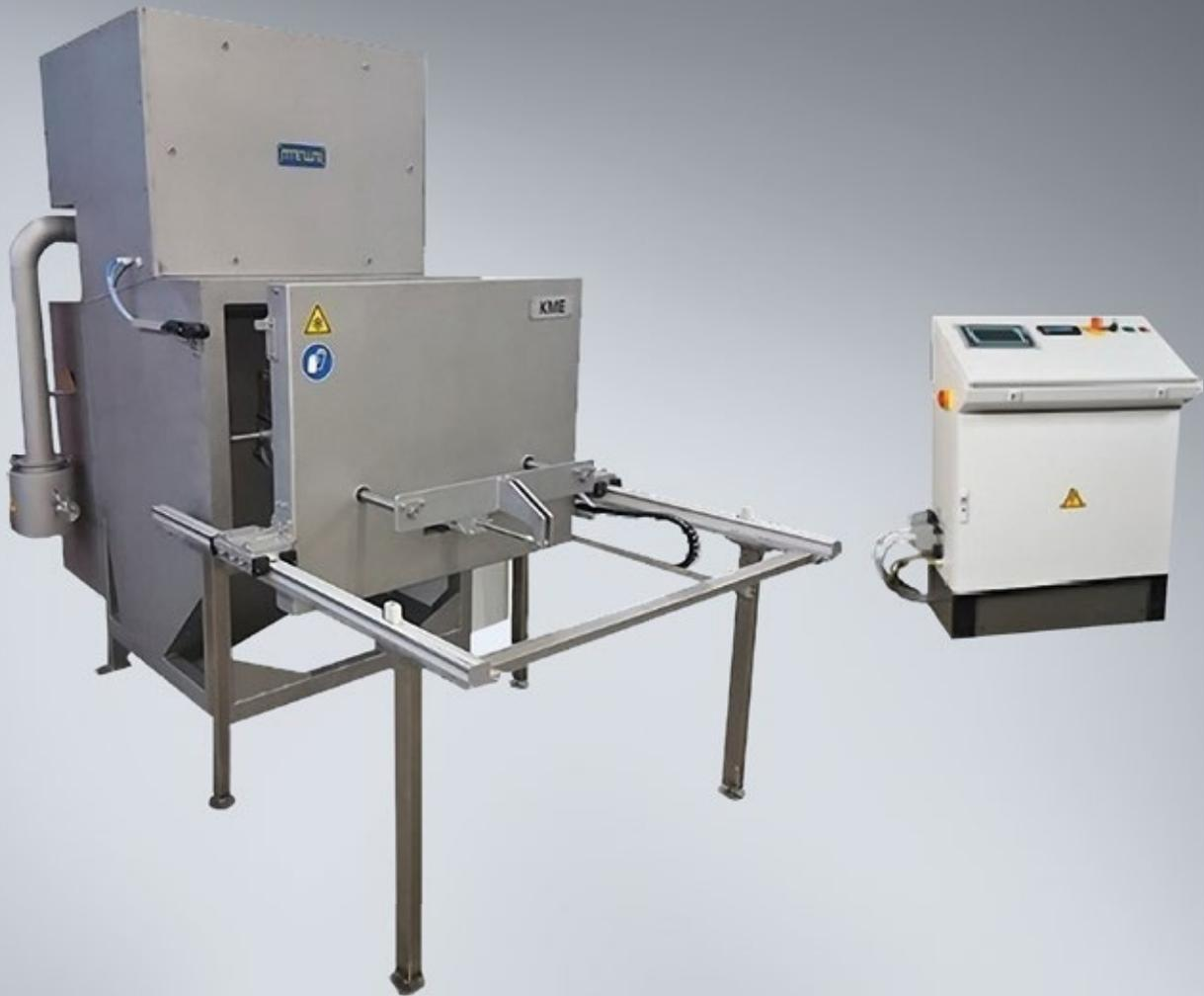
**The KME system is a high-performance deburring system for various cryogenic deburring applications of molded parts made of rubber, plastics and non-ferrous metals with a length of up to 500mm with quick-change basket system.**
