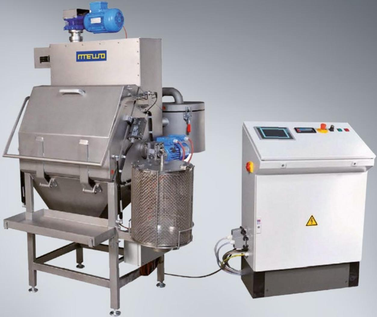
**The TS 7.12 is a high-performance compact media-blasting deburring system for various cryogenic deburring applications of seals and moulded parts made of rubber, plastics and non-ferrous metals.**
